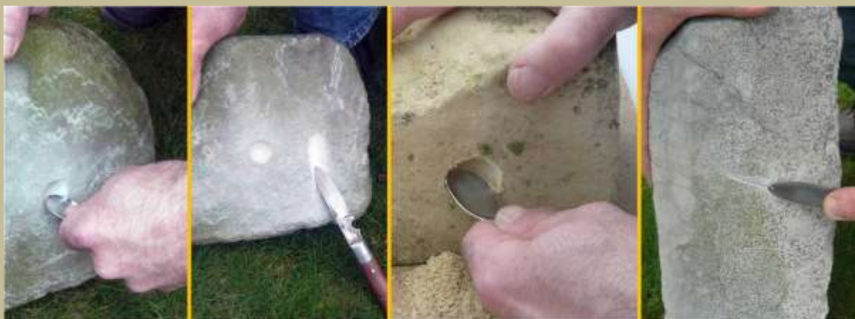
Experimenting with making scratch marks in Bentheimer sandstone (photo 1 + 2), in limestone ('marl', photo 3) and in lower carboniferous limestone (photo 4)
